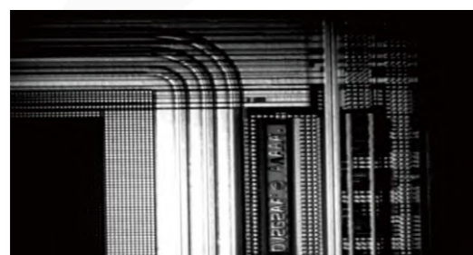
Non-destructive analysis of bad chip packaging
